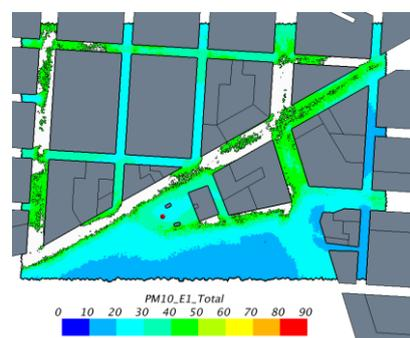
Fig.1 Average PM10 concentrations ( $\mu\text{g}/\text{m}^3$ ) at 3 m above ground level for the period January-March 2011 considering road traffic and boiler emissions and the background concentration. Areas with concentration higher than 50  $\mu\text{g}/\text{m}^3$  are in white.
