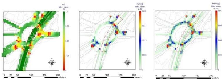
*Fig1. Average speed,  $\text{NO}_x$  and  $\text{PM}_{10}$  emission distribution for free flow conditions*
